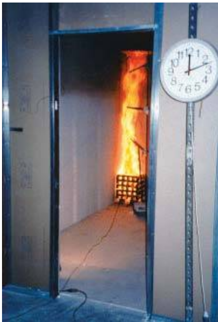
Actual fire rating test on Perform Wall After four hours test was halted – wall is impervious to fire, water, insects and mold
